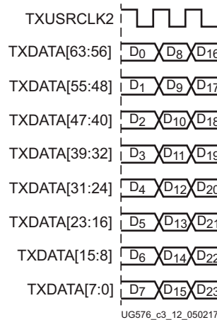
Figure 3-12: Input to the 8-Byte to 4-Byte Converter (TX_DATA_WIDTH = 64 (8-Byte), TX_INT_DATAWIDTH = 1 (4-Byte), GEARBOX_MODE[2] = 1'b1)
